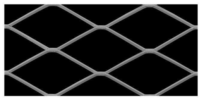
LW Pitch:85.73mmStrand Width:3.18mmSW Pitch:40.64mmThickness:3.00mmWeight:3.67 kg / m2Open Area:84%
